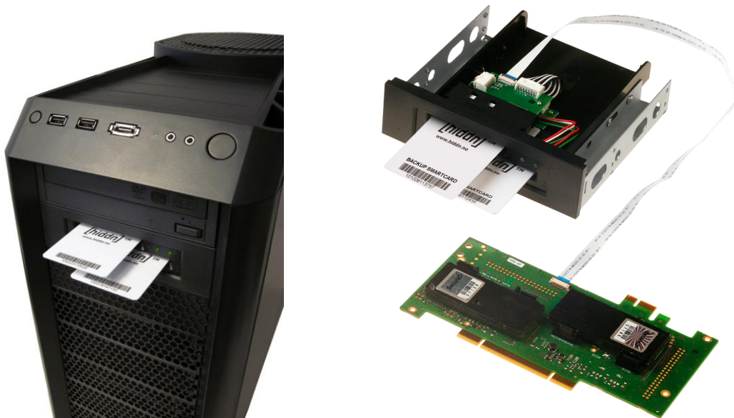
Figure 9 [hiddn]™ Desktop – installed and “out of box”
