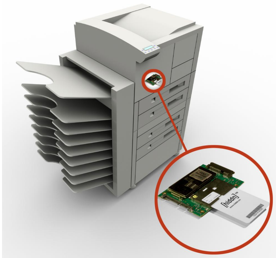
Figure 12 [hiddn] ™ SATA Adapter – conceptual installation in copier
